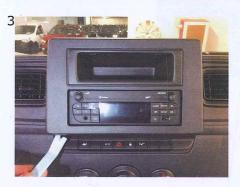
3 Remove the OEM facia plate as shown in the picture.
