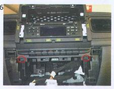
6 Unscrew and save the 2 screws circled in red. Remove the keys panel. Disconnect and remove the radio from the radio tunnel
