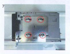
7 Fix the mounting brackets to the radio by tightening the 4 screws for side circled in red.
